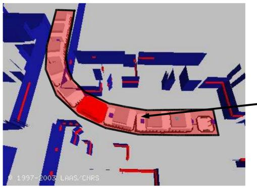
collision tunnel for body trailer swept volume =  $w_{trailer} + 2\rho$
